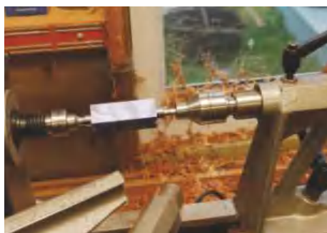
▲ Pic.4 Mount the blank onto the mandrel with the correct bushings for the kit
